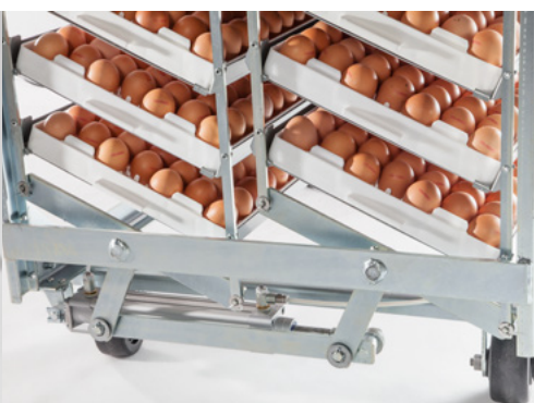
Individual air piston on each incubator trolley
