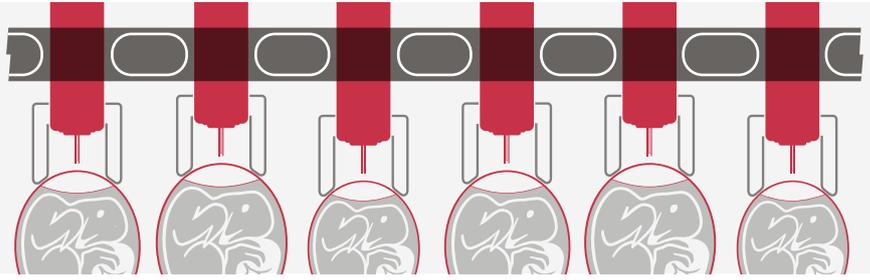
**2** Special air tubes between the injectors inflate, locking the injectors in the ideal position. The injector head then makes a second fixed, downward movement, causing the injector's outer needles to pierce the shell collectively and precisely.
