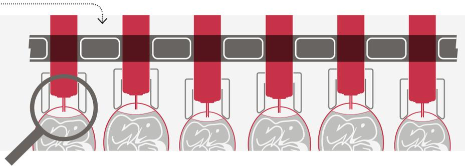
**3** To allow automatic and individual adaptation of the injection depth to each single embryo (regardless of egg size and flock age), the inner needles in each injector then descend individually.
