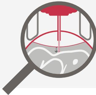
**5** The Embryo Soft Touch® sensor detects the position of the embryo and the needle movement stops. Retracting slightly to avoid any injury to the embryo, the inner needle remains in the amniotic fluid.
