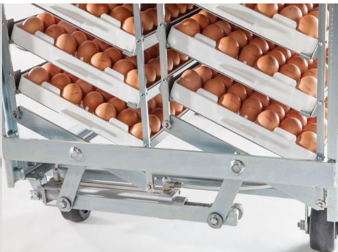
Individual air piston on each incubator trolley
